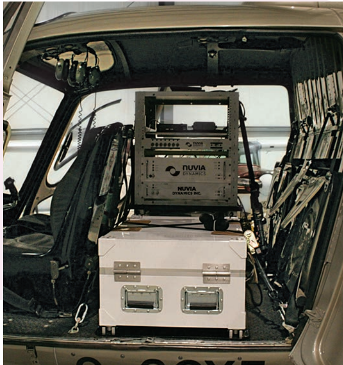
AGRS-5 installation in AS350 helicopter for integrated system test flight in Canada.
