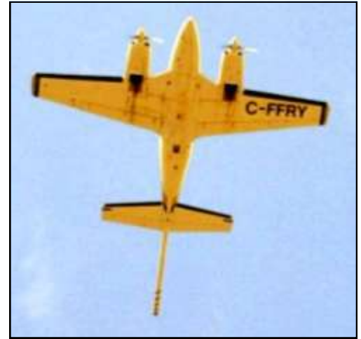
Piper PA31 Navajo Survey aircraft featuring a high-sensitivity cesium magnetometer and an AGRS gammametry spectrometer with 33.6 litres of GSX sensor in the aircraft's cabin
