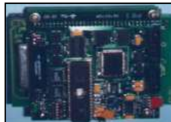
DPD-1 Digital Peak Detector in PC-104 format
