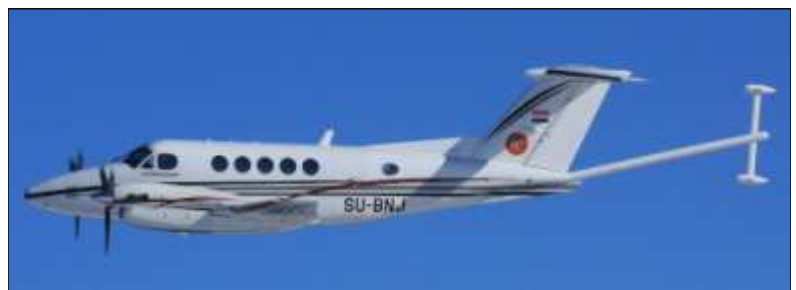
AGRS with three GSX-1024/256 Gammametry spectrometer sensors is installed in this Beech B200SE King Air survey aircraft
