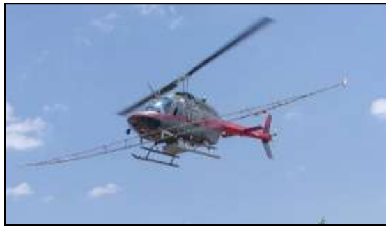
A helicopter-borne (Bell 206B3 Jet Ranger) horizontal magnetic gradiometer system with a GSX-1024/256 sensor installed in a rack underneath the forward part of the cabin
