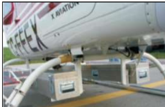
Two GSX-HeliSPEC Gammaray Detectors installed on a Bell 206L Long Ranger helicopter for a total of 16.8 litres of detector.
