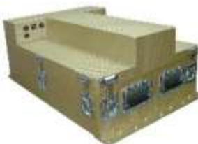
An AGRS-10S advanced gammaray spectrometer system was part of the airborne system. It included 4 of these GSX-1024 sensors with a total of 50 litres of detector
