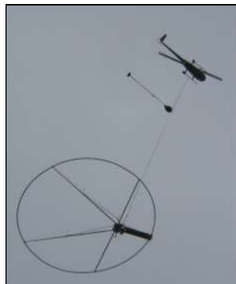
P-THEM-Lite lightweight time domain EM system in flight with a Robinson R44 Raven helicopter
