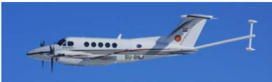
NMA's modified and newly painted Beech B200SE King Air aircraft undergoing its flight testing in Canada
