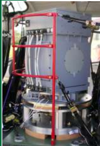
The AMSE GT-1A installed in an Eurocopter AS350B2 helicopter in Toronto for flight and acceptance tests
